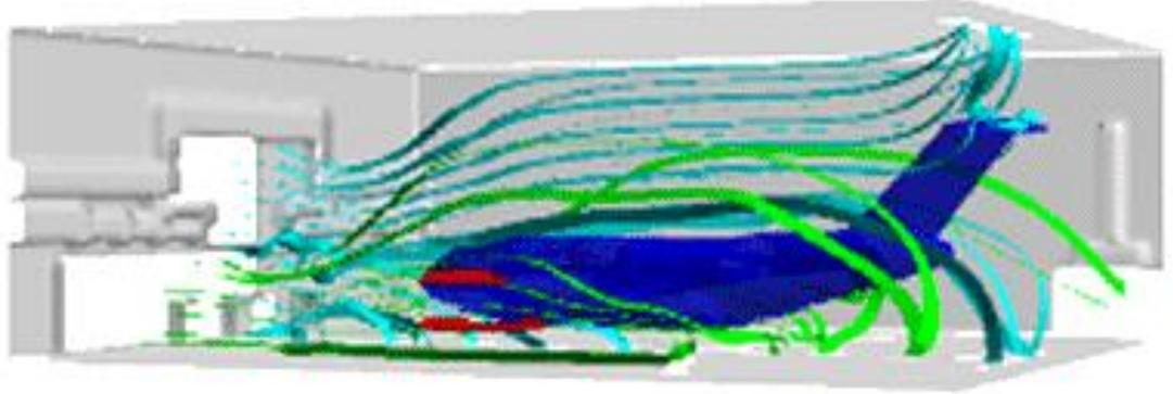
The modeling analysis addressed the airflow, air balance, and operation of the supply air exhaust systems, including the requirements for the supply air and exhaust air plenum segments.
