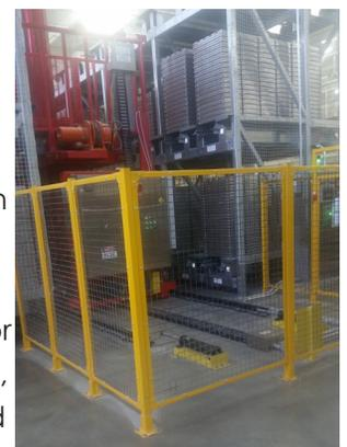
10. Basket stacking – Manual basket stacking is also challenging labor that results in many back injuries. Automated basket stacking and unstacking eliminates this issue. Automation here may be a large investment up-front, but systems are reliable and pay for themselves through labor savings and injury reduction.
